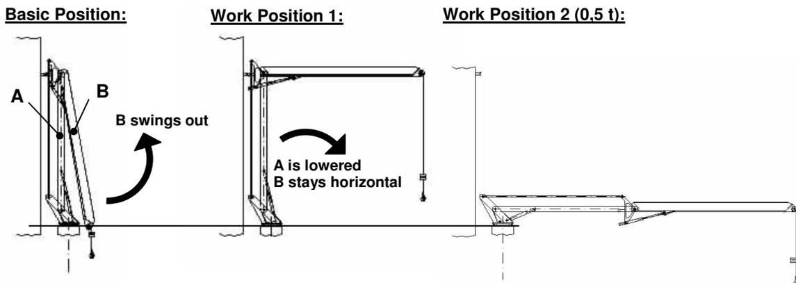
**Fig. 4: Various working positions of the PTS**
