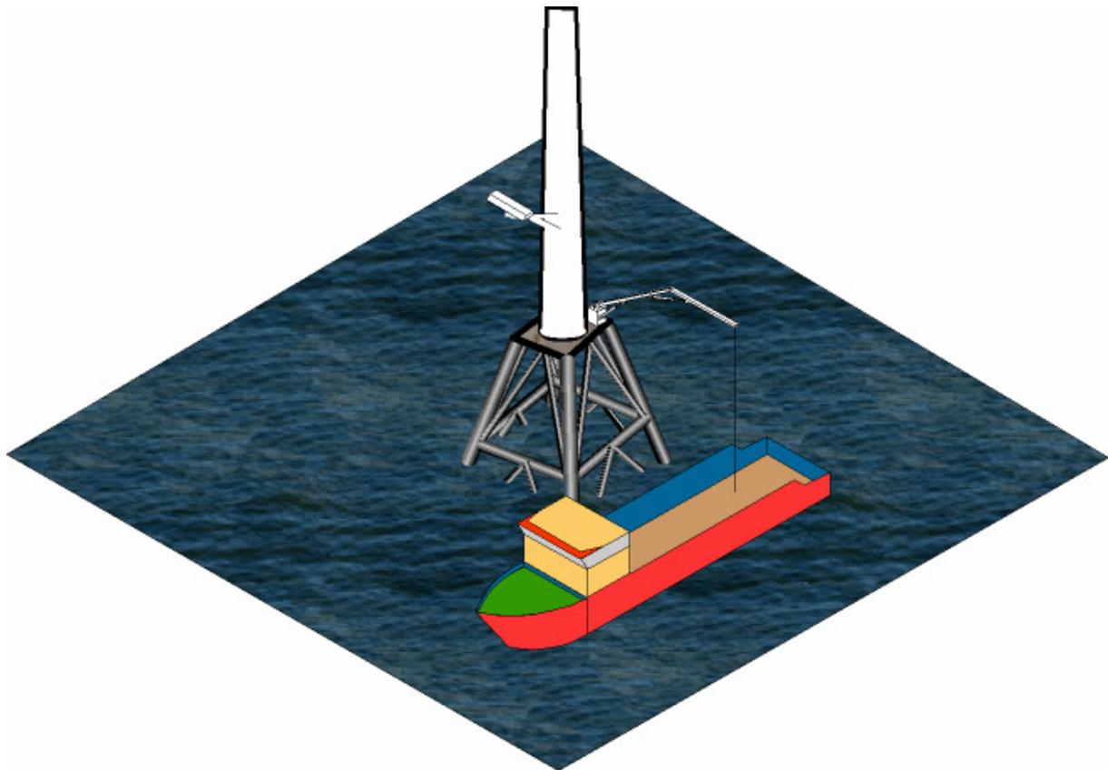
**Fig. 3: Schematic Picture of the Personnel Transfer System Inclusive Service Vessel**
